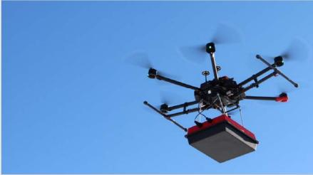
Drone Plug-In GPR with low frequency SE-model antennas Designed for very deep geololgical applications 5 kg payload. 10-80 m depths – meter resolution.
