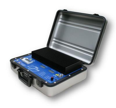
The terraTX-50 base unit comes complete with the console, battery pack (designed to hold 2 x 12V batteries), battery charger, 5m synchronisation cable, loop input cable, 7m couput cable, console power cable, three battery interlink cables, and an operation manual on CD. Optional enhancements available for use with the terraTX-50 include a 200m synchronising cable supplied on a reel to be used in place of the 5m synchronisation cable.
