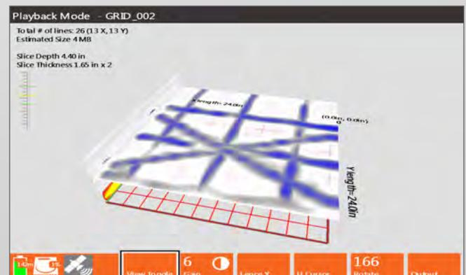
Screen capture of 3D data image. Data illustrates a rebar mat with post tension cables in an "X" pattern.
