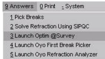
The Optim analysis is a velocity optimization. It uses the first break picks to repeatedly forward model the subsurface. Numerous test velocity models are created, through which travel times are calculated and compared to the observed data. The model that has the smallest discrepancy with the observed data is selected for the final output.
