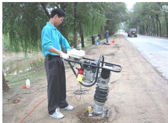
Inexpensive construction tampers are used as the energy source. Picture from Langfang, China.
