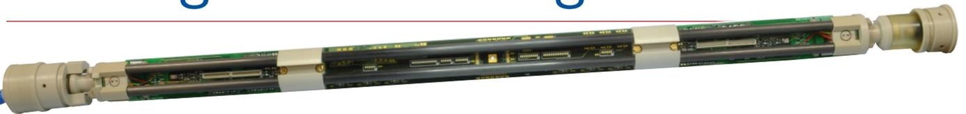
The new Grad-13 will be available from Bartington Instruments in summer 2013, for use in UXO detection on land, underwater, and in boreholes.
