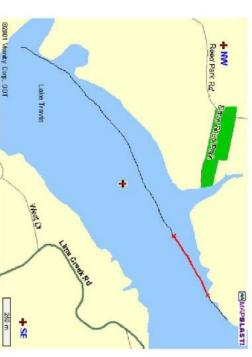
the total path run, the red line shows the extracted used to plot the survey line. The black line shows resistivity profile in the resistivity image above. The Marine Module of the Administrator software is
