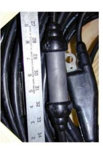
passed through it. The towing cable that it does not corrode as current is has a kevlar member and water block. (patent pending), the advantage is The sea electrode is made of graphite
